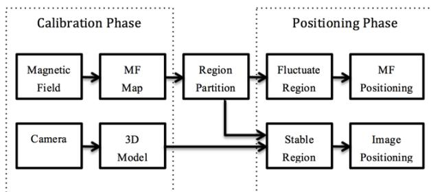
Fig. 4. Whole process of the proposed localisation method
