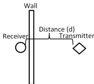
Figure 2. Bluetooth Transmitter, Receiver, and Obstruction Arrangement.
