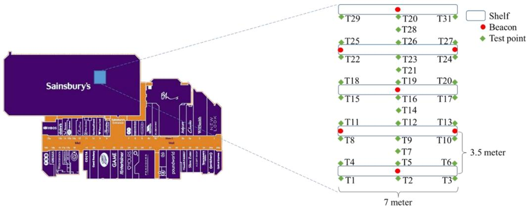
Figure 9. Beacon and Test Points Layout at Cameron Toll Shopping Mall.
