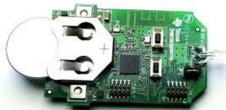
Figure 1. Bluetooth Low Energy Beacon CC2540DK-Mini.
