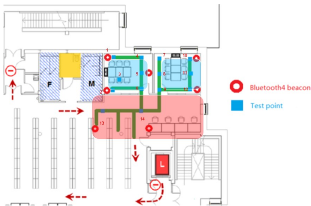
Figure 9. Layout for BLE beacons in the library (7 beacons)
